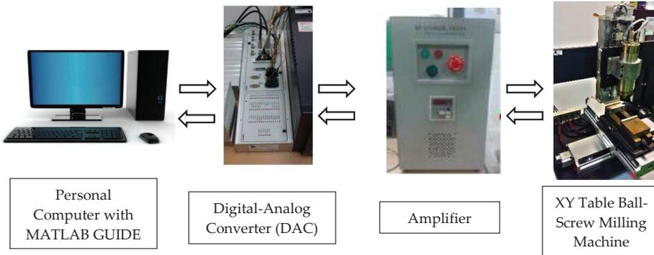
Figure 2: Experimental setup of XY table ball-screw driven system
