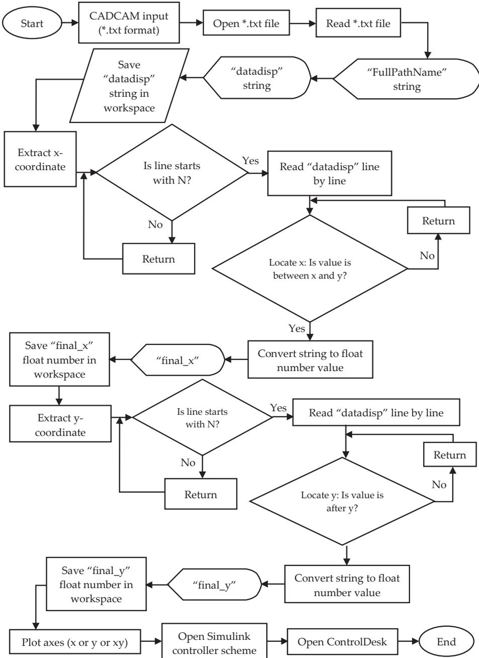
Figure 4: Workflow of CS-DES interface system
