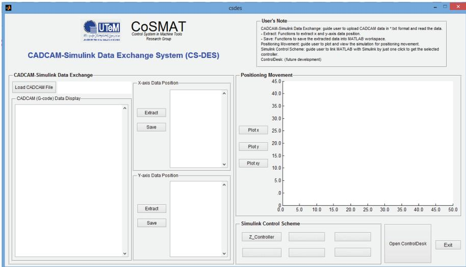
Figure 3: The developed CS-DES interface system
