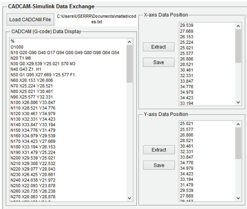
Figure 6: Example of extracted  $x$ -axis and  $y$ -axis positions data
