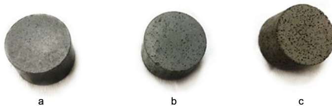
Figure 2: Physical observation of (a) green part, (b) brown part and (c) sintered part
