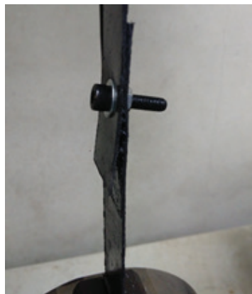
Figure 5: Secondary bending effect observed for CQ4 hybrid SLJ
