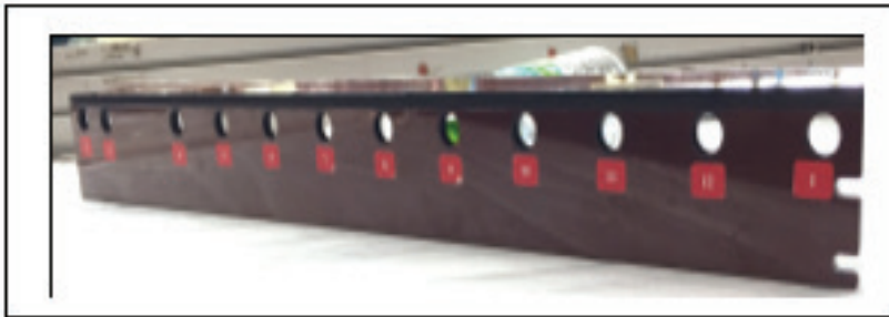
Figure 3: Point to point checking jig
