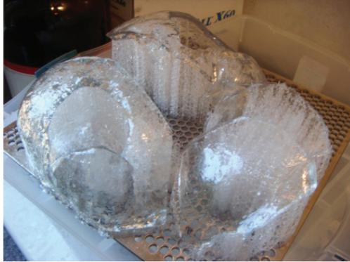
Figure 7: Completed SLA parts before the cleaning process
