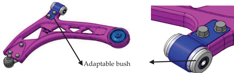
Figure 10: Final design of aluminum cast FLCA with adaptable bush
