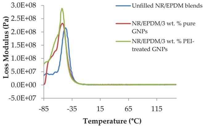
Figure 3: Loss modulus of unfilled NR/EPDM blends and NR/EPDM filled GNPs nanocomposites
