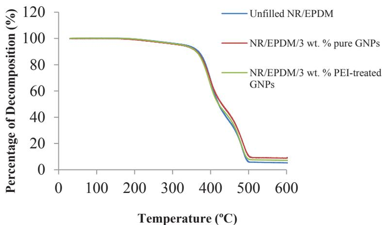
Figure 5: TGA curves for unfilled NR/EPDM blends and NR/EPDM filled GNPs nanocomposites
