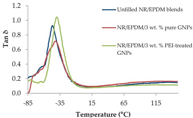
Figure 4: Tan  $\delta$  of unfilled NR/EPDM blends and NR/EPDM filled GNPs nanocomposites
