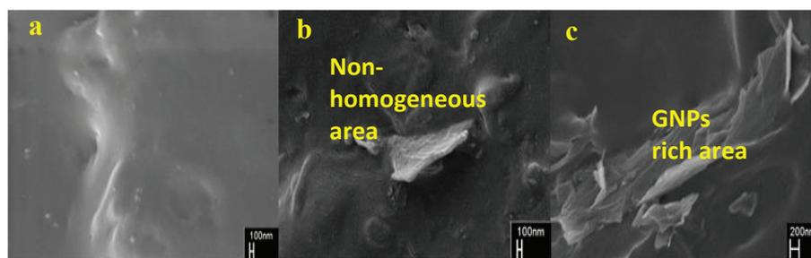
Figure 7: Fractured surface morphology of (a) unfilled NR/EPDM blends, (b) NR/EPDM blends filled with 3.00 wt. % PEI treated GNPs, and (c) NR/EPDM blends filled with 5.00 wt. % PEI treated GNPs
