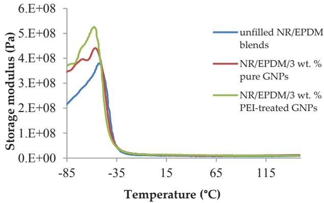
Figure 2: Storage modulus of unfilled NR/EPDM blends and NR/EPDM filled GNPs nanocomposites
