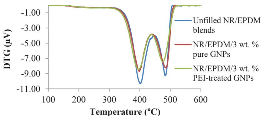
Figure 6: DTG curves for unfilled NR/EPDM blends and NR/EPDM filled GNPs nanocomposite
