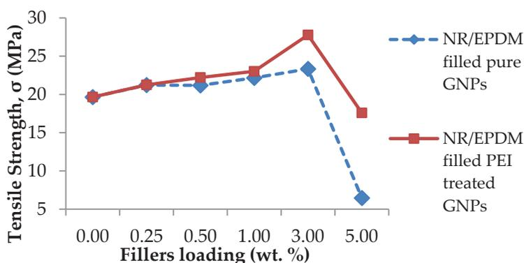
Figure 1: The effect of GNPs loading on the tensile strength of NR/EPDM blends filled with pure GNPs and PEI treated GNPs (A: NR/EPDM filled pure GNPs nanocomposites; B: NR/EPDM filled PEI treated GNPs nanocomposites)
