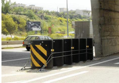
Figure 2.3: Crash block make from smart plastic (HMW/HDPE) (Google.com, 2011).
