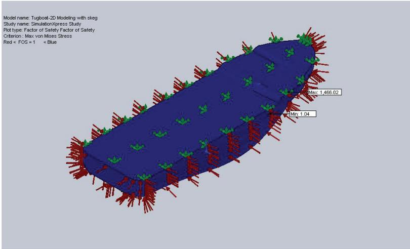
Figure 15: Result of Factor of Safety
