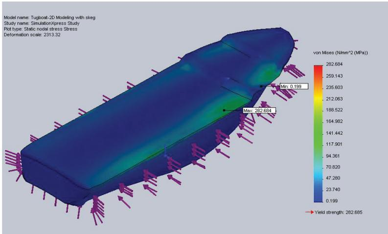
Figure 12: Result of Von Mises Stress (Equivalent Stress)
