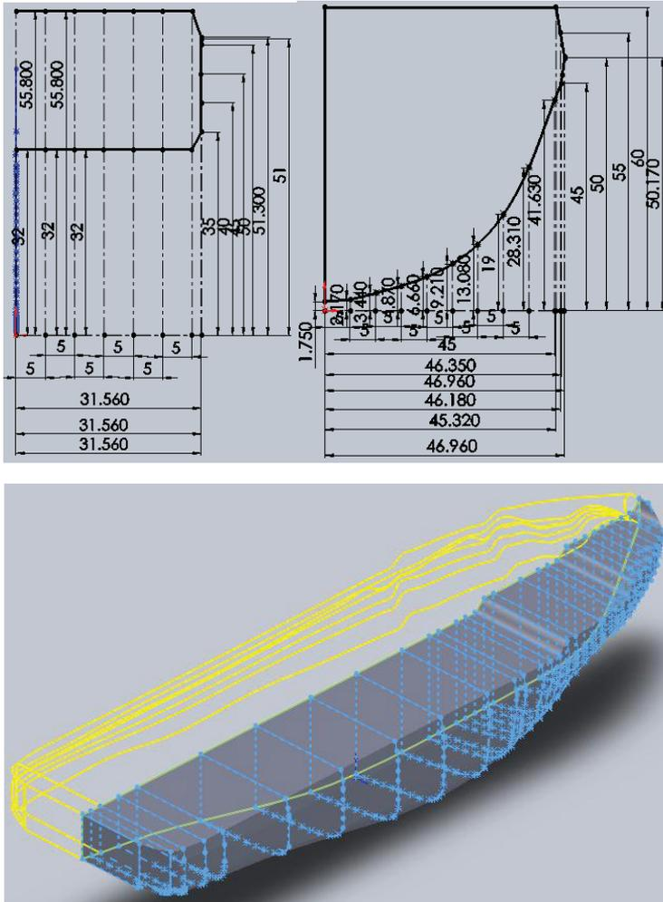
Figure 4: 3D Structural System of Bollard Pull Harbour Tug
