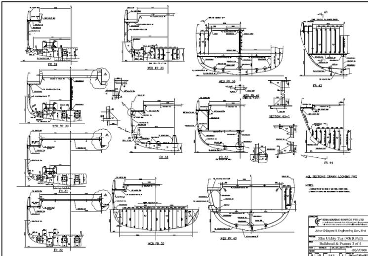
Figure 3: 2D Structural System of Bollard Pull Harbour Tug
