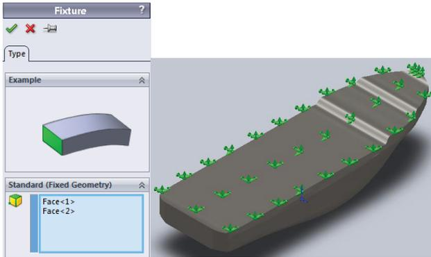
Figure 5: Fixture Setup on the Upper Surface
