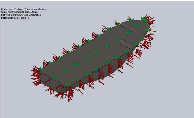
Figure 14: Result of deformation
