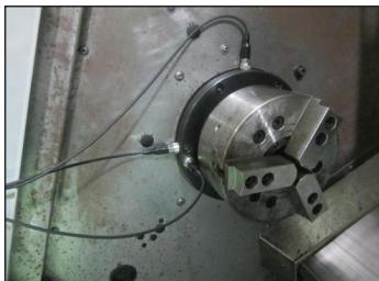
Fig. 2a. Accelerometer in 3 axes location
