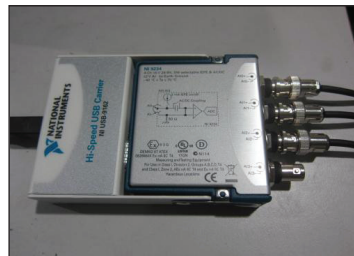
Fig. 2b: The high speed USB centre connecting the accelerometer and PC
