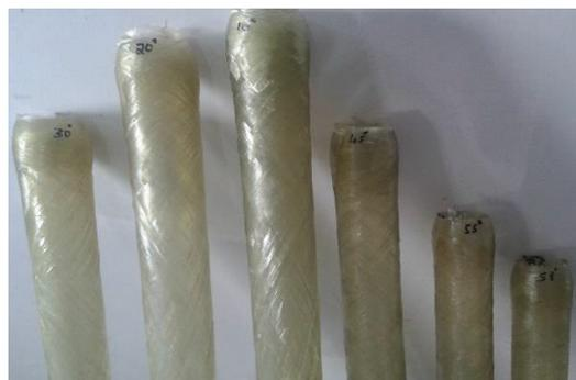
Figure 6: Filament wound pipe
