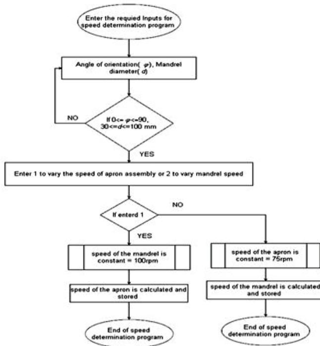
Figure 3: Speed determination sequence
