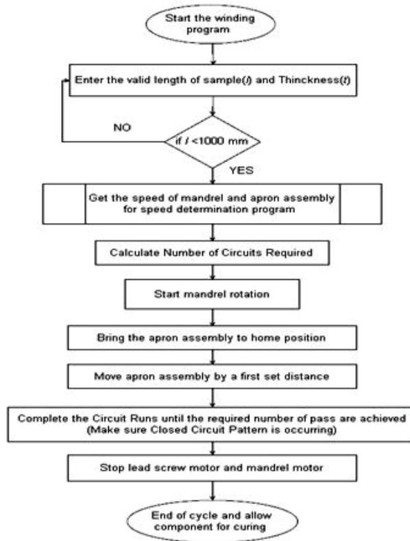
Figure 4: Winding sequence
