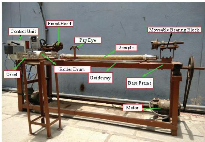
Figure 5: Filament winding machine
