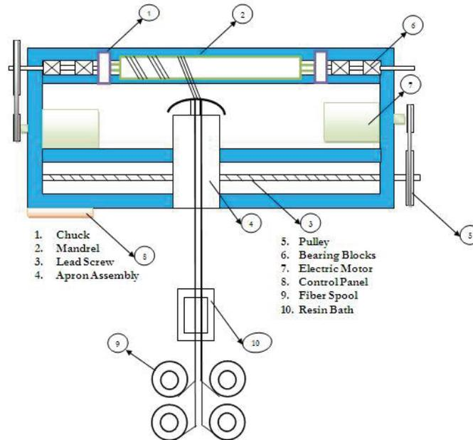
Figure 1: Schematic diagram of proposed filament winding machine
