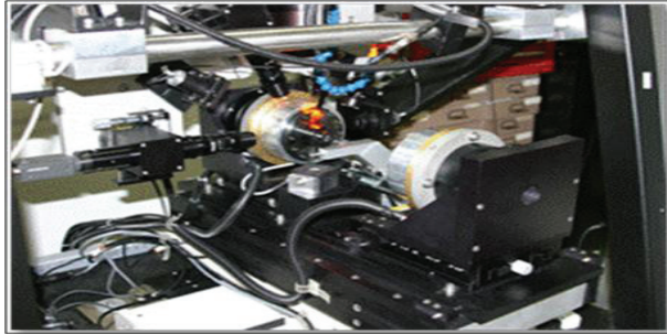
Figure 1: Shows the existing laser lathe system. ( www.resonetics.com/pages/LaserTechnology )
