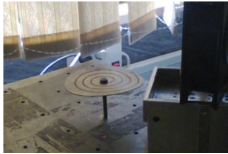
Figure 13: Spiral exposure on sheet metal
