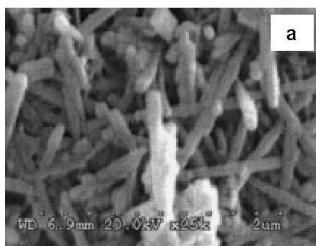
Figure 3: HA crystals at the same temperature 140°C of different pH, (a) pH 9 and (b) pH 14 (Liu, et al. , 2003).
