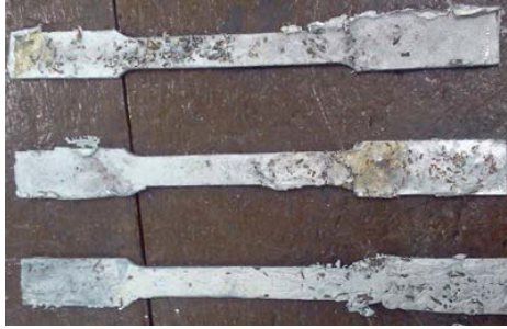
Figure 8: Uneven distribution of rice husk and SiC
