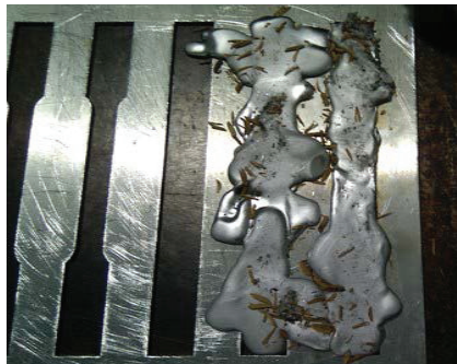
Figure 3: Solidified molten mixture inside the open mould
