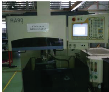
Figure 2: WEDM model MITSUBISHI RA 90
