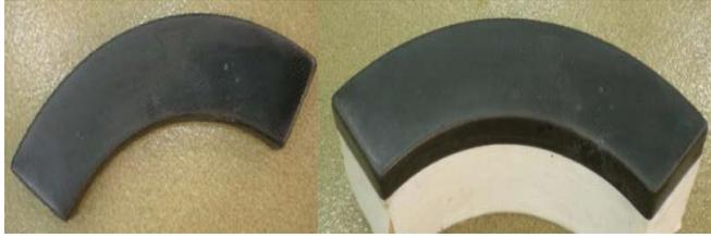
Figure 8: C shaped RIDFTed multiscale laminates infused with 1 and 2 wt% CNT doped vinyl-ester resin
